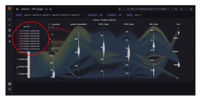
In the above image, data for a single node has been highlighted using the top-left panel.
